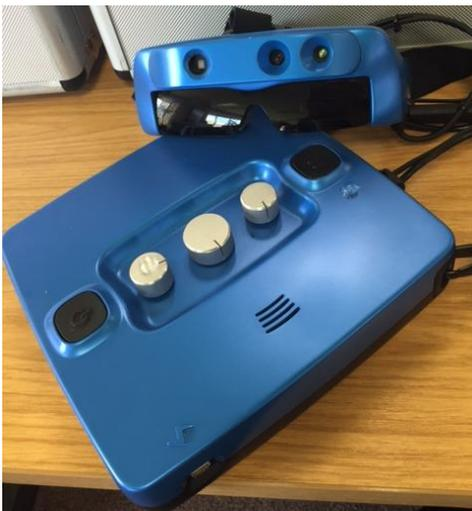
The Smart Glasses unit is made up of a headset and a control box which are connected by a cable. The Smart Glasses allow the user to change between five ‘modes’: the first two modes use an infra-red camera and show the world in monochrome. These modes are most useful for low or indoor light. The last two modes use a regular (visible light, RGB) camera and can therefore be used outdoors. Mode 3 uses data from both cameras. Only
